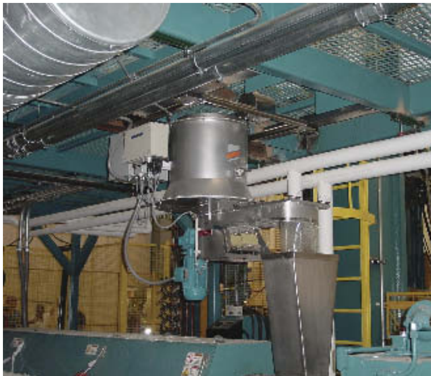
The resonant-frequency feeding system incorporates a hopper with a bottom agitator, a vibratory feed tray, a loss-in-weight weighing system, and controls.
