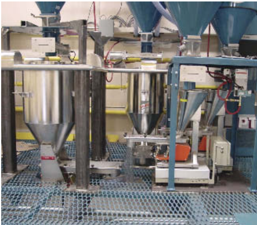
The tray feeder uses the supplier’s patented vibration technology to provide a specified feedrate without breaking down or degrading the fiberglass.
